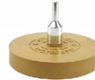
ITEM NO. ERP88 / ERP102 Thickness: 15mm Ø 88mm Thickness: 20mm Ø 102mm Thread 5/16" -24(Including a drill adaptor) Max.RPM: 4000
