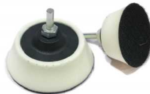
ITEM NO. MS-DPB03-50 2" (Ø50mm) ITEM NO. MS-DPB03-75 3" (Ø75mm) PU Thickness: 20mm Thread M6
