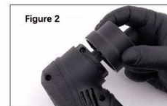
Then install protection cover as shown in figure 2.
